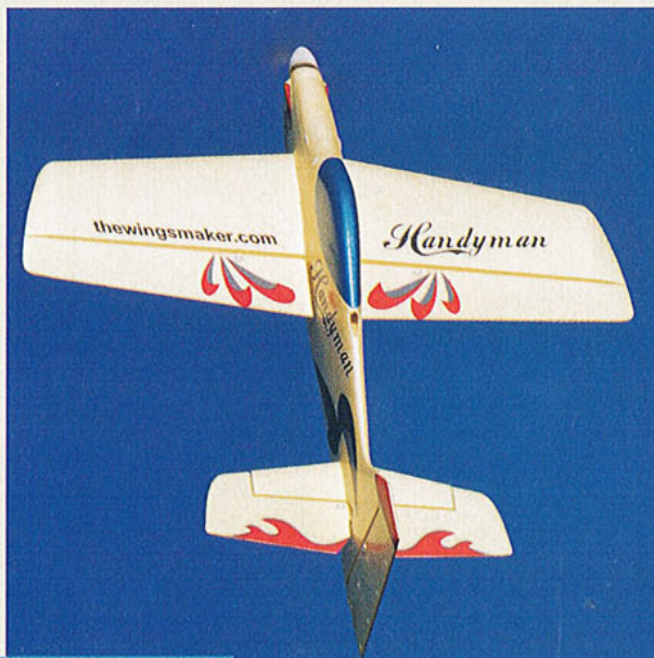
The Handyman goes into and maintains a hover quite easily. I might add some more aileron throw to prevent it from torque-rolling out of the hover when the throttle is bumped up. It flew just as well in the inverted attitude as it did right-side-up.
