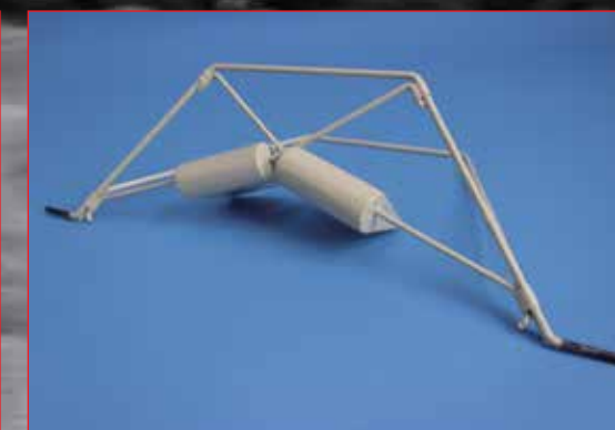
The main gear has some beautiful, airfoil-shaped, imitation bungee covers that add some extra pop to the scale looks of the plane.
