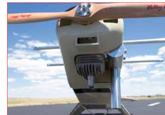
▲ The DLA-56, gas-powered engine fits the fiberglass cowl perfectly. I used the vacuum-formed plastic cowl template to mark the fiberglass cowl for cutting.
