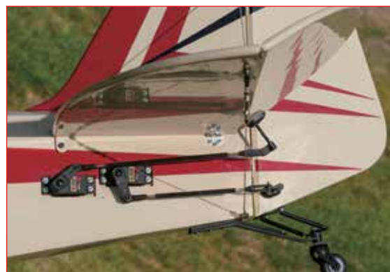
The servos for the elevators and rudder are easy to install in the aft end of the fuselage. It is a well-engineered design that provides positive control.
