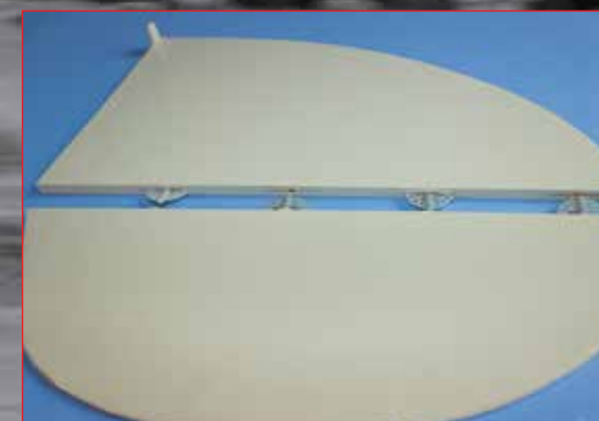
The supplied hinges and pre-cut slots are a huge time saver when it comes to building the elevators, rudder and wings.
