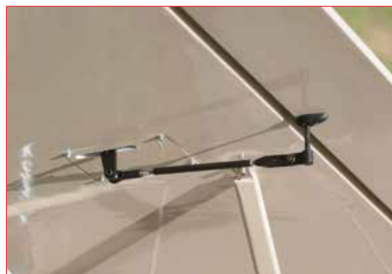
In this photo you see how the servos get installed in the wings for aileron control. Again, it is a clean and well-engineered design that makes for excellent control.
