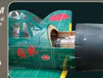
Detachable battery hatch for easy access to battery compartment
