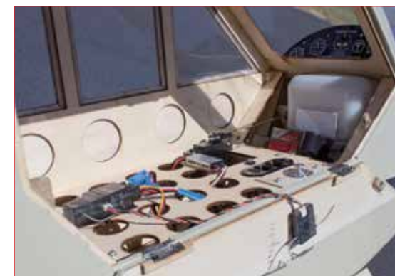
▲ The electronics fit perfectly in the bottom servo tray and keep everything out of sight when the pilot tray is installed in the cockpit.
