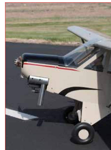
▲ This shows you another angle of how the fiberglass cowl gets cut to fit the DLA-56 engine. It makes for a very clean engine installation in the model.
