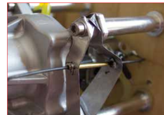
▲ I made my own guide for the choke rod from an old spray can of brake cleaner and a piece of brass tube.
