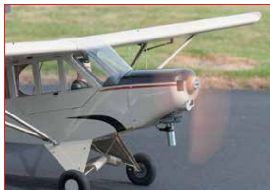
▲ World Models provides a pilot for the cockpit. The landing gear struts are well built and include the scale bungee fairings that you would see on a full-scale.
