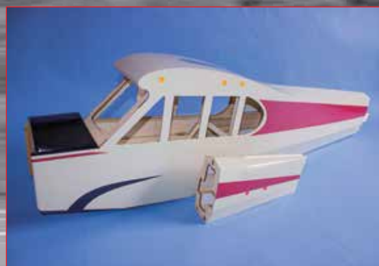
Those little orange and red dots are your opening locators for the fuselage and tail section.
