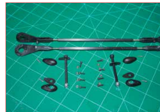
▲ The supplied hardware comes with ball bearings to reduce binding in the control rods.
