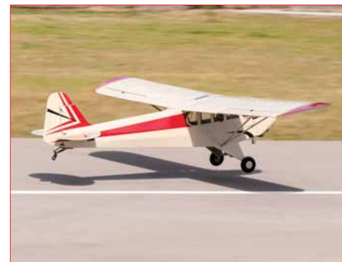
You will discover that when you apply the throttle the model's tail will start to fly almost from the minute the airplane start rolling.
