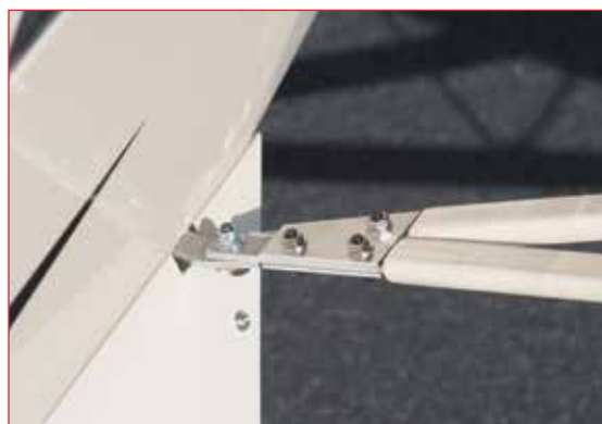
▲ The wing's struts get attached to the fuselage by way of a bolt and lock nut. You'll find that it will only take a few minutes to assemble this model.
